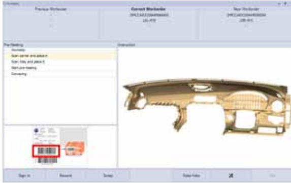
Figure 3: HYDRA Dynamic Manufacturing Control guides operators on the Dynamic Line Panel
