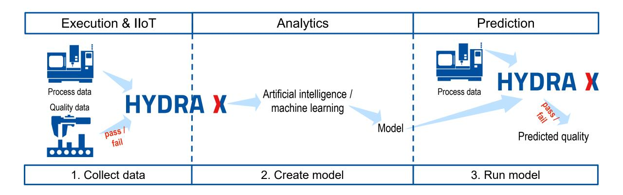
Predictive Quality can forecast product quality during manufacturing based on current process values and an AI model.
